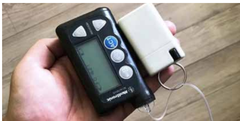
Kamil's set-up, showing the pump and the RileyLink, which communicates between the pump and the smartphone
